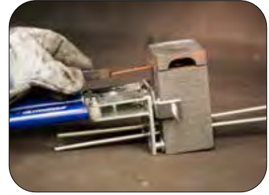
Step 3: Close the lid and attach DRONE cord to the UltraShot igniter.
