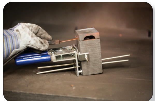
step 3 Close the lid and attach DRONE cord to the UltraShot® igniter.
