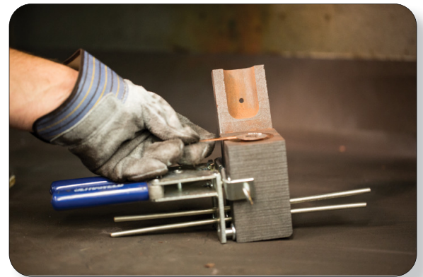
step 2 Place conductors and UltraShot® cartridge into mold.
