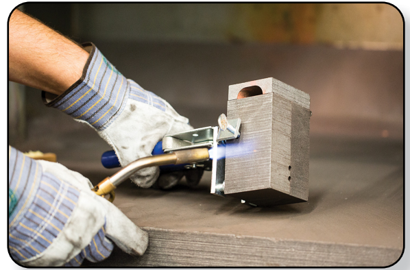
step 1 Dry and Clean the mold and conductor.
